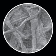
Ultra High Efficiency media is designed to meet the need for a greater level of filtration and dirtholding capacity. Cat UHE Air Filters feature a unique surface that extends filter life up to
