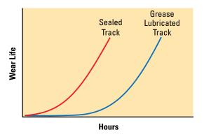
With Grease Lubricated Track, internal wear is eliminated until the grease dissipates from the line assembly. Wear begins immediately with Sealed Track.
