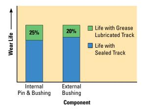
Increased wear life of pin and bushing means more sprocket and link life is utilized.
