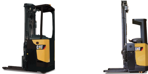
Stacker range: 1.0 – 2.0 tonne capacity
