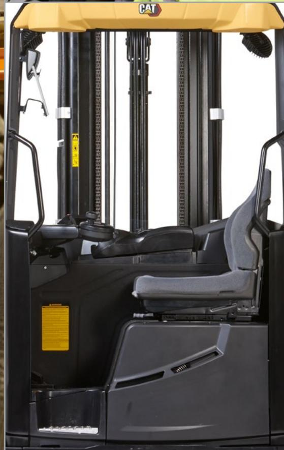
Exceptionally clear operator's view (left and below), with carefully placed cables and hoses and incorporation of hydraulic cylinders into the mast profile (far left).
