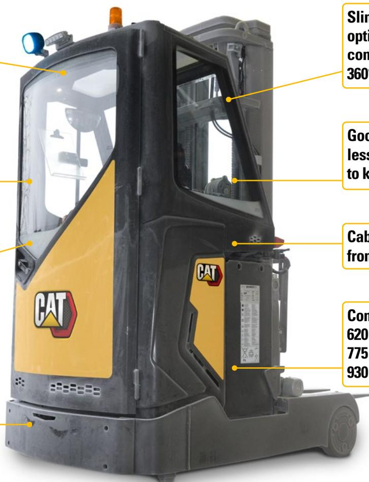
When equipped with both the cabin and the necessary cold store modification (MODCS), a reach truck can operate dependably in freezing temperatures as low as  $-35^{\circ}\text{C}$ .
